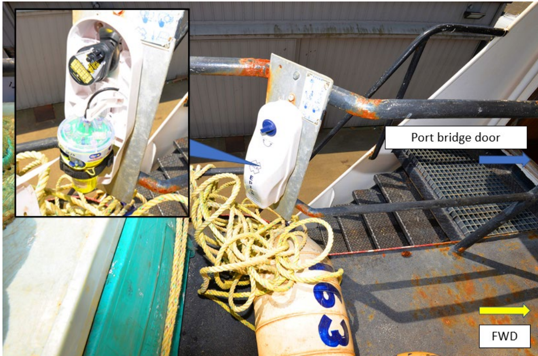
Figure 14. The Scandies Rose EPIRB mounted on the handrail aft of the bridge. Inset shows the float-free EPIRB with protective cover removed.
