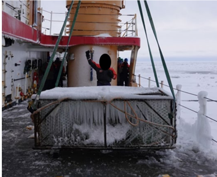
Figure 23. Crewmembers aboard USCGC Polar Star weigh a crab pot following a 3-day freezing spray experiment.
