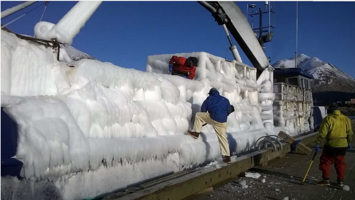
Figure 24. Ice accumulation on the fishing vessel Sandra Five in King Cove, Alaska, February 12, 2017. The vessel was operating the previous day in the Bering Sea in the vicinity of the Destination (NTSB 2018).
