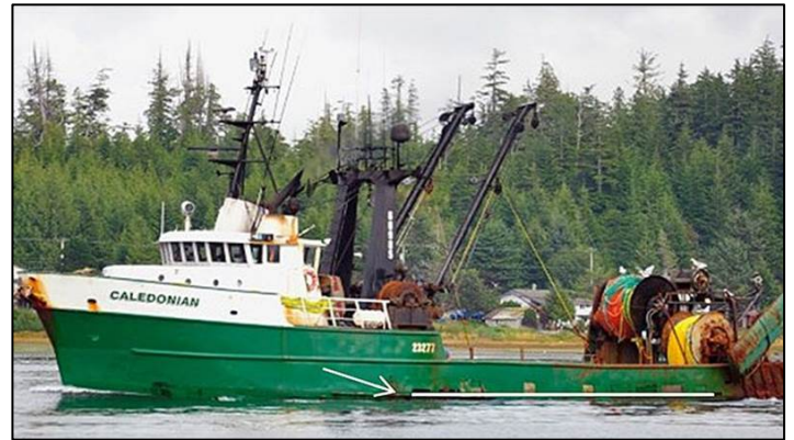
The Caledonian in loaded condition; white line indicates her deck level (credit TSB / Eric Sorenson)
